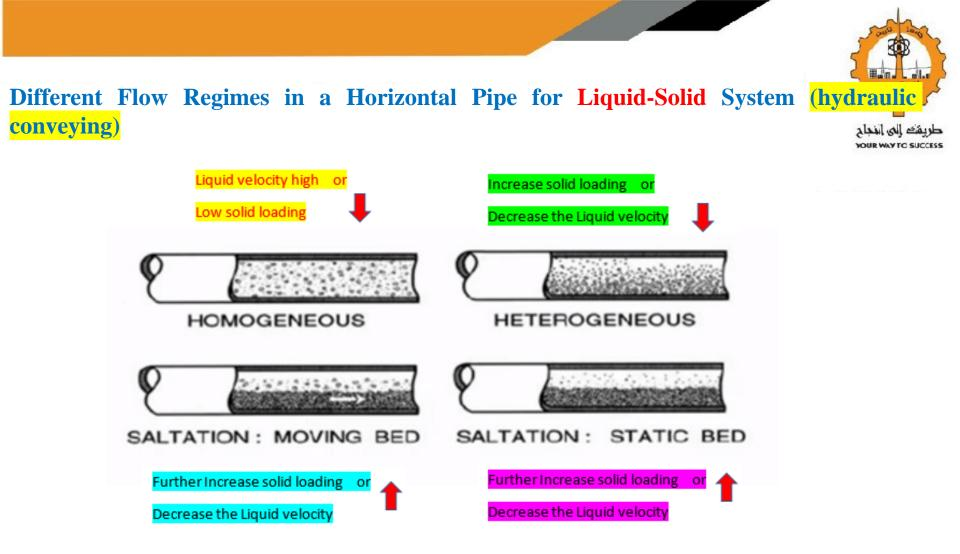
Flow regimes for liquid-Solid slurry flow in a horizontal pipe
